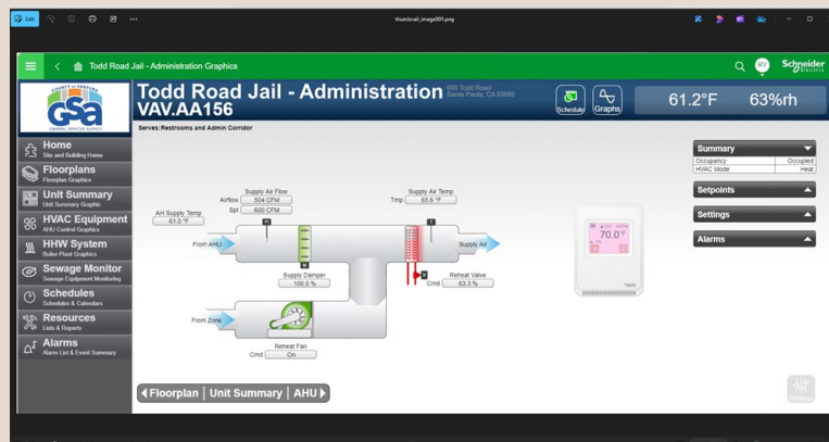
Sample screenshot of County's Energy Management System (EMS) used by GSA F&M to manage HVAC system assets.
